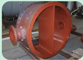
water-box and distributors lining
