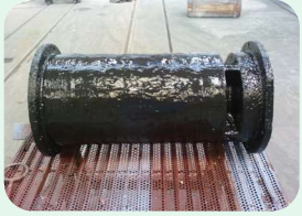
refurbishment of heavy pitted surface
