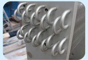
antibacterial coating of HVAC equipment
