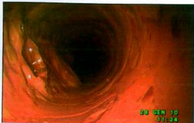
FIG. 23 Tubo esercito con blistering. Inner tube blistering after service.
