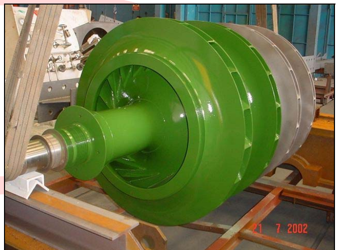
Compressor rotor: ceramic filled high-solid abrasion resistant coating.
