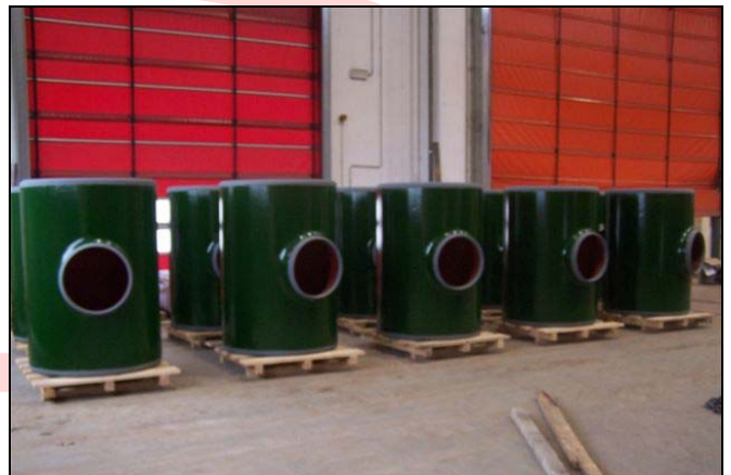
Pipelines coated with hot spray applied, high-solid, solvent-free, self-priming epoxy amine cured material.
