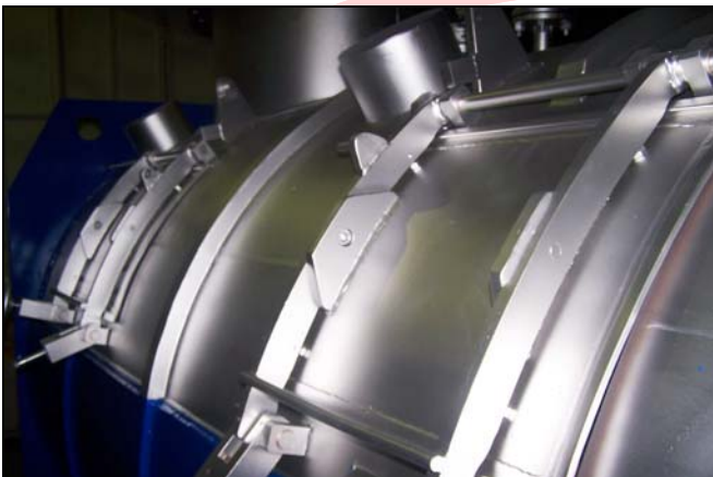
Stainless steel surface after glass abrasive blasting to provide smooth finish.
