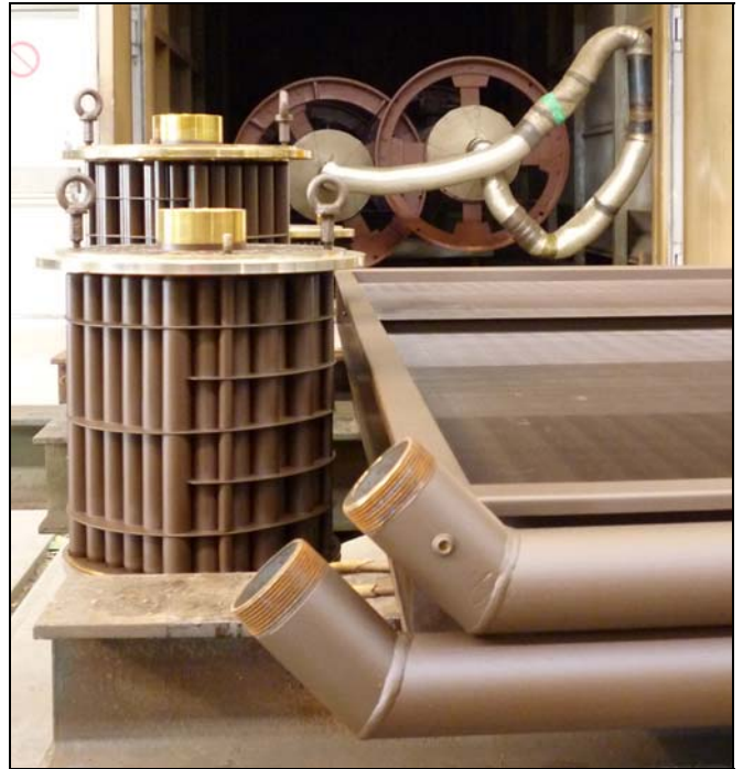
A finned pack heat exchanger, various removable bundles and 2 shell-tube heat exchanger prior curing (back).
