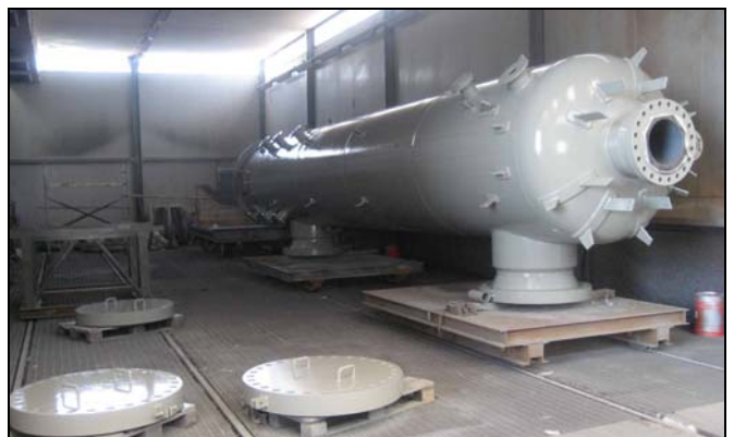
External and internal coating of contactor.
