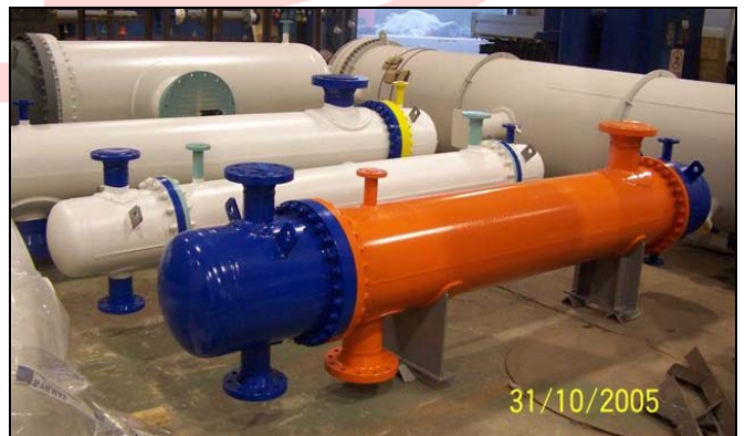
Vessels and filters coated with different painting systems.
