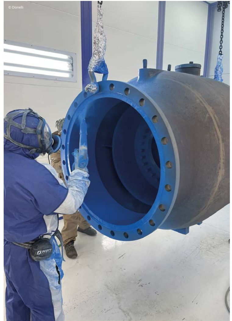
FBE powder coatings call for higher thicknesses than conventional powders.
