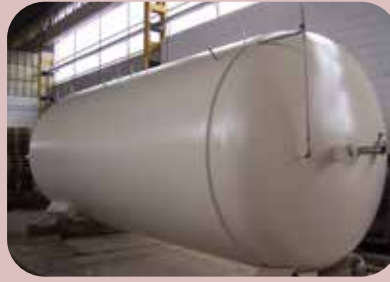
external coating of tanks
